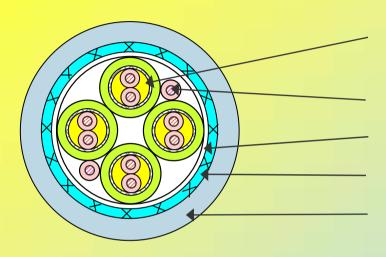
Twisted pair with shielding and jacket
